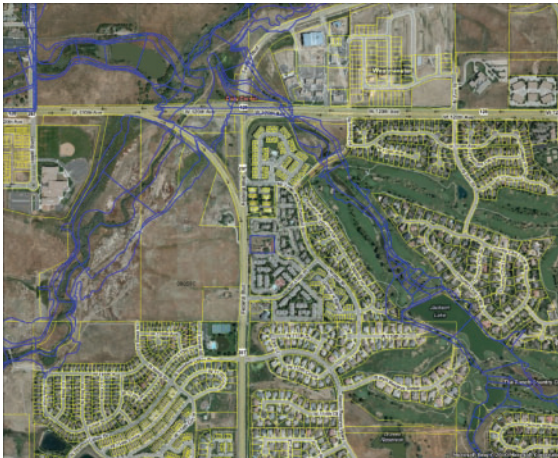
Figure 1. A parcel-centroid level view of a subdivision shows both property boundaries (in yellow) and flood areas (in blue)
